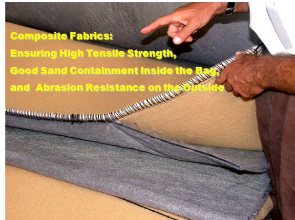
Figure 4.33: Material used for large sand bags
