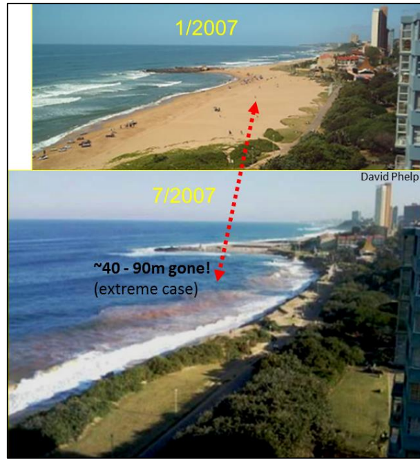
Figure 4.9: KZN example of extreme shoreline erosion along an exposed location (Phelp et al, 2009)
