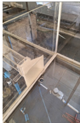
FIGURE 6: Culvert model showing 3D printed inlet
