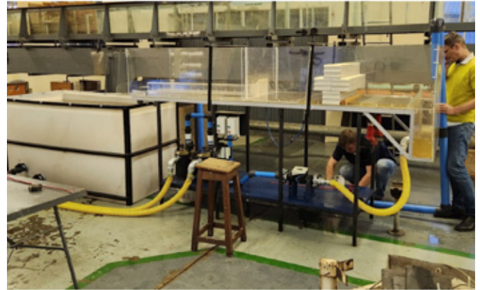
FIGURE 5: Physical model (flume with culvert model)
