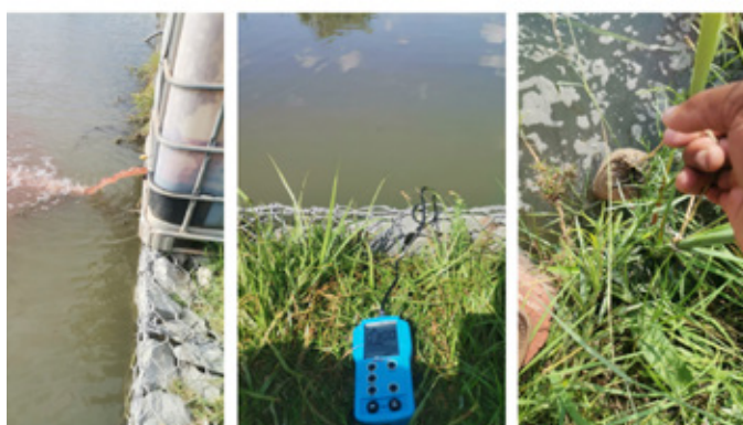
FIGURE 6: Showing dosage of microbes – liquid form and in bacbag, real time testing of pH, conductivity, temperature, suspended solids sampling water from the lake during monitoring process.
