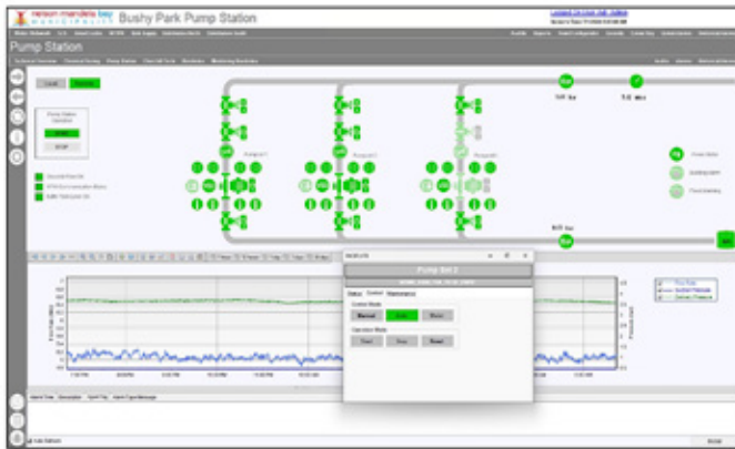
FIGURE 12: Screenshot of the NMBM's Bushy Park pump station SCADA system with pumpset number 2's faceplate shown.
