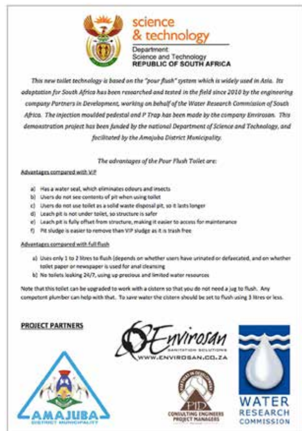
FIGURE 7: Piloting and Testing by the Department of Science and Technology
