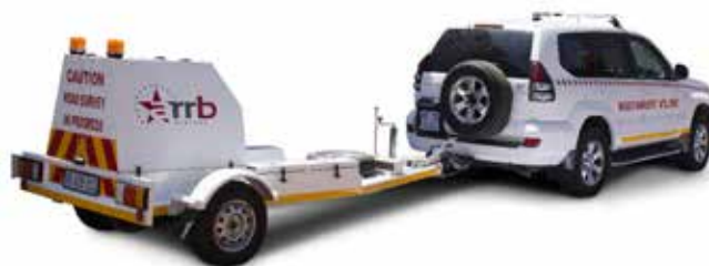
FIGURE 8: Falling Weight Deflectometer and towing vehicle
