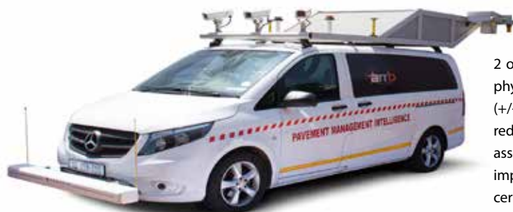
FIGURE 6: Network Survey Vehicle incorporating LCMS
