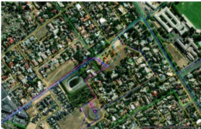
FIGURE 2(B): Detailed view GIS representation of different pipe diameters from the Drakenstein hydraulic model
