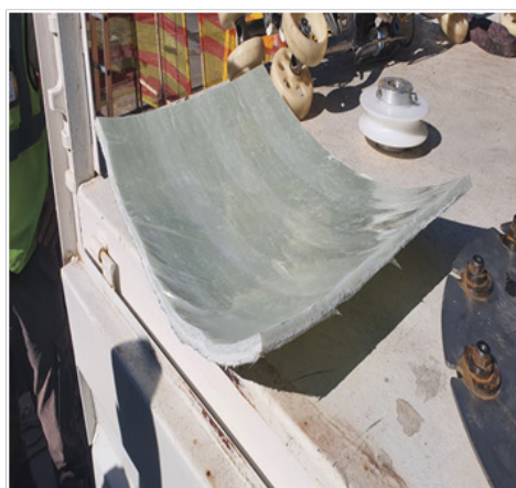
FIGURE 28: Sample of CIPP liner cut out for testing after curing
