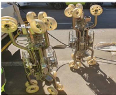
FIGURE 22: UV Light train on site
