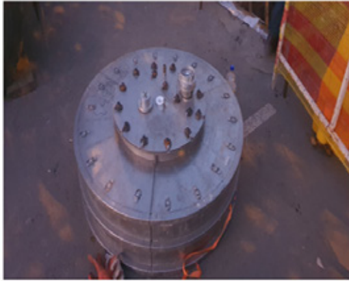
FIGURE 20: Folding packer with pressure nozzles for inflating the liner
