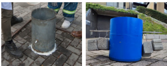
FIGURE 2: ASTM C1781 test apparatus (left) and Mod-ASTM test apparatus (right)
