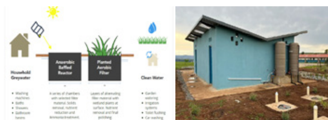
FIGURE 5: DewDrop Recycle Toilet Process (Left) and Demonstration (Right)
