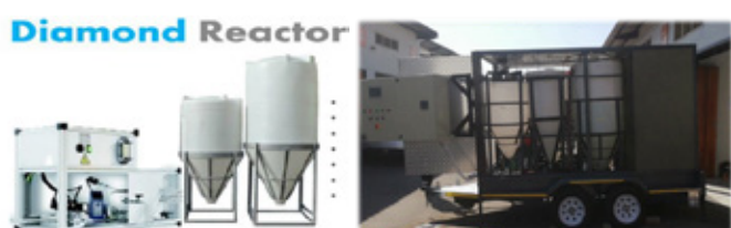
FIGURE 8: Struvite Reactor Units
