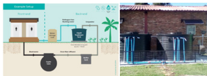
FIGURE 4: Aquonic Recycle Toilet process (Left) and Demonstration (right)
