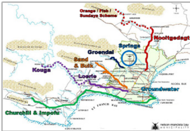
FIGURE 3: Diagrammatic layout of NMBM's Bulk water systems
