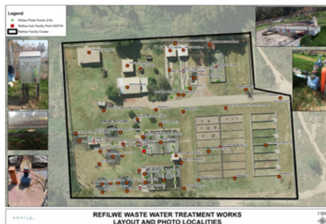
FIGURE 8: Example of geographic representation of the asset components and geo-referenced locality of the photographic records
