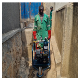
FIGURE 6: A portable vacuum pumping machine such as the Pitvaq is useful for suction pumping in places where vacuum tankers are either not available, or unable to access the site.
