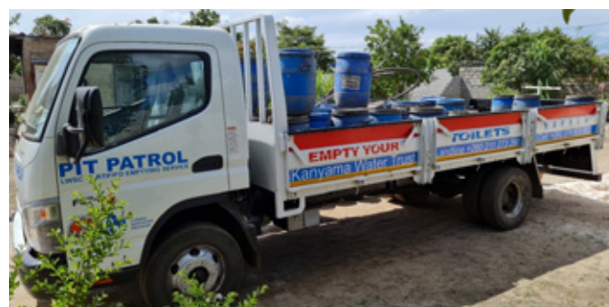
FIGURE 7: Pit emptying contractors in Lusaka, Zambia, use a combination of manual/mechanically assisted emptying and vacuum tankers. When they empty pits manually they use drums which are sealed and transported by truck.
